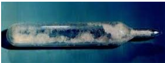
Fig. 11: (b) UF 6 in a glass ampoule. Source: web.ead.anl.gov/uranium/guide/UF6
